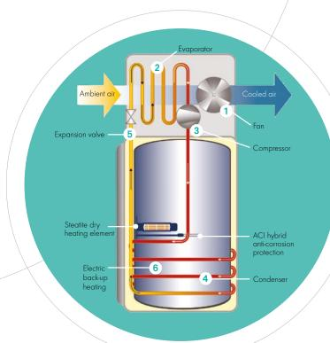
EXPLORER'S TANK AND HEATING ELEMENT:
